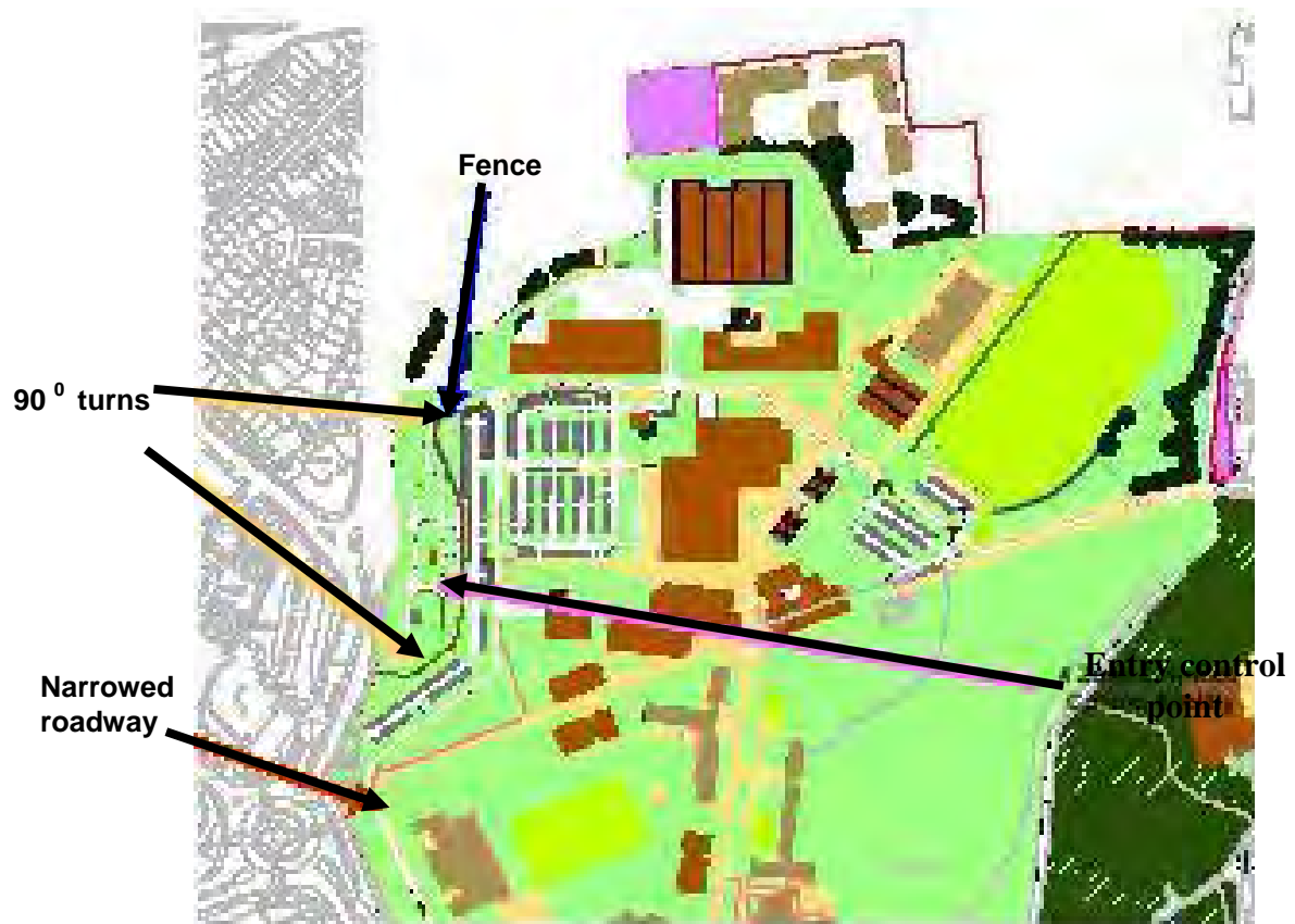
Figure 5-3. Road Modifications to Reduce Speed
